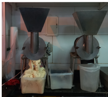
Figure 2. Electric mill for preparing acarajé and abará batter.
